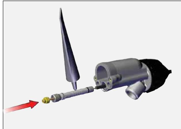
2. Tighten packing using wrench. Pull back and forth on the needle shaft till a slight amount of drag is felt.
