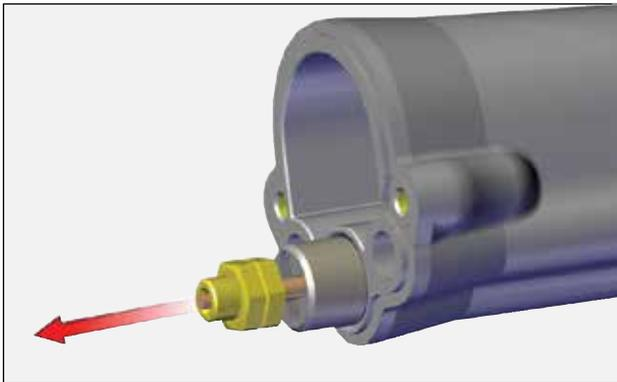
4. Remove jam nuts using 10mm wrench.
