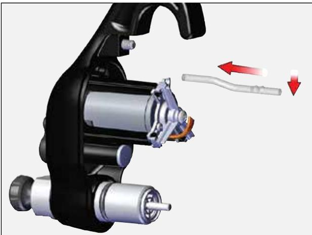
6. Install fluid valve cartridge.
