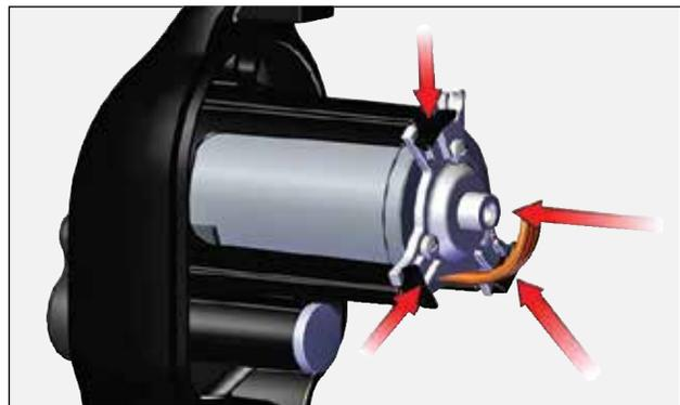
3. Install cartridge then o-ring (if removed).
