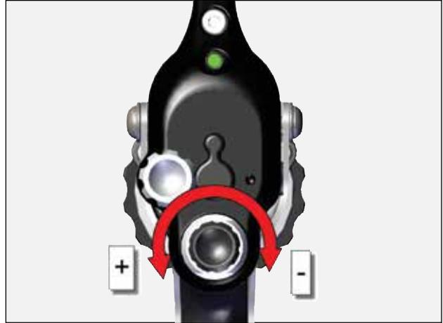
15. Adjust compensation valve with small driver.
