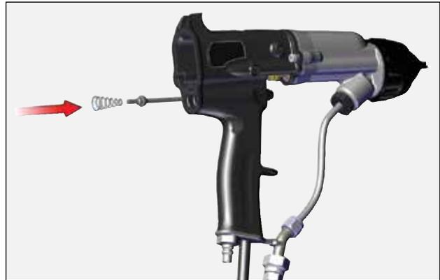
6. Tighten packing nut till light drag is felt on the shaft while moving it back and forth.
