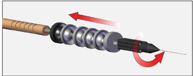
8. Insert packing tube onto shaft. Wipe excess grease over front parts and outside of packing tube.
