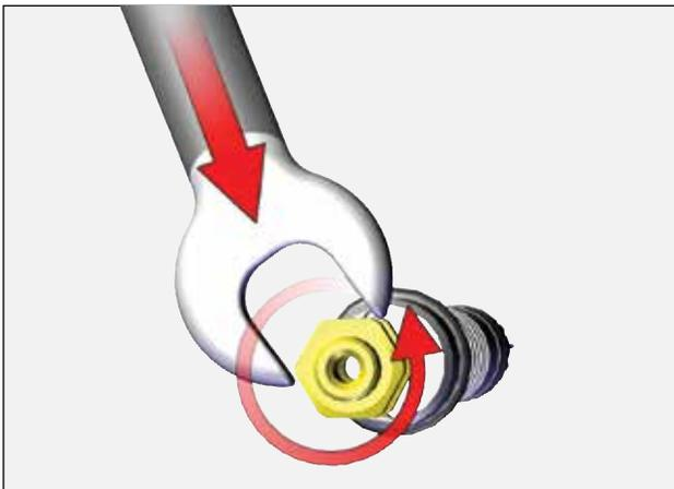
5. Remove all parts, clean with non-polar solvent. Inspect for any discolored areas. Replace parts as required.
