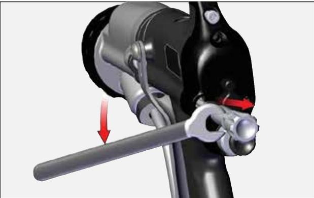
3. Remove rear cover and cartridge with 15mm wrench.
