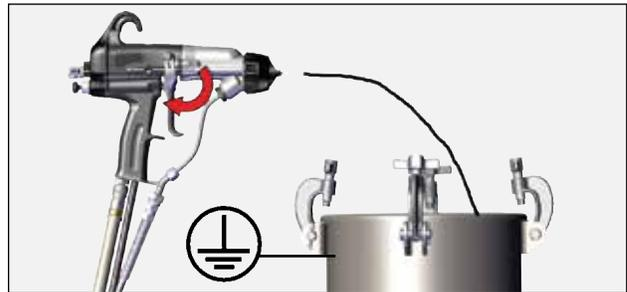
4. Release trigger stop material flow.
