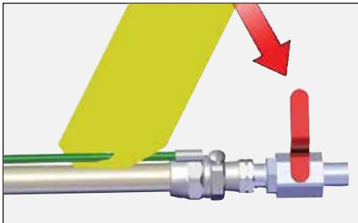
3. Discharge fluid into appropriate earth grounded metal container
