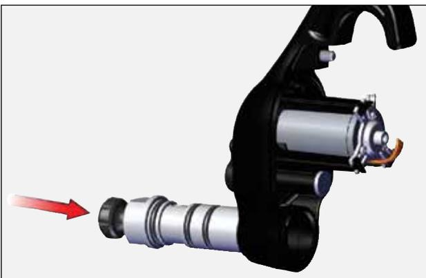
7. Install gasket and re-connect motor connector to handle harness connector.
