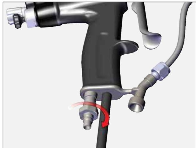
3. Remove bracket, gasket and o-ring.
